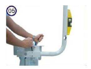
(05) After leveling, adequately tighten the 4 screws (A). Use an allen key type 5/16" and a wrench 9/16".
