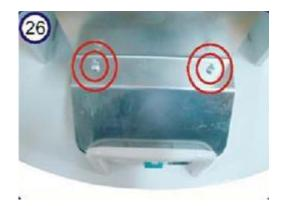
(26) Replace the PCB's protective cover and the screws. Use a Philips screwdriver.
