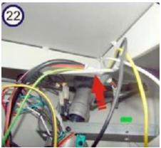
(22) On the front and back part of the chair, pass the light's wire through the supporting passage.
