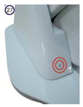
(27) Replace the housing cover and the screws (left and right side). Use a Philips screwdriver.
