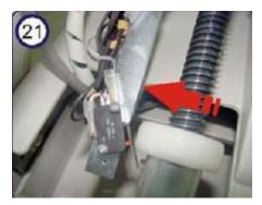
(21) Pass the light's electrical wire over the cover of the actuator.
