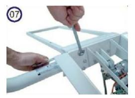
(07) Mount the frame to the seat, setting it through the 2 hex bolts with flat washers and nuts. Use two fixed wrenches 9/16".
