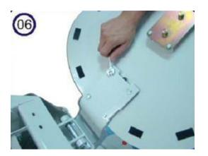
(06) Mount the back plate and secure it through the 4 hex bolts with flat washers. Use a wrench 7/16".
