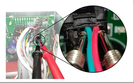
Turn the potentiometer wheel until you read 4.0 VDC +/- .1v. Reinstall the belt onto the pully.
